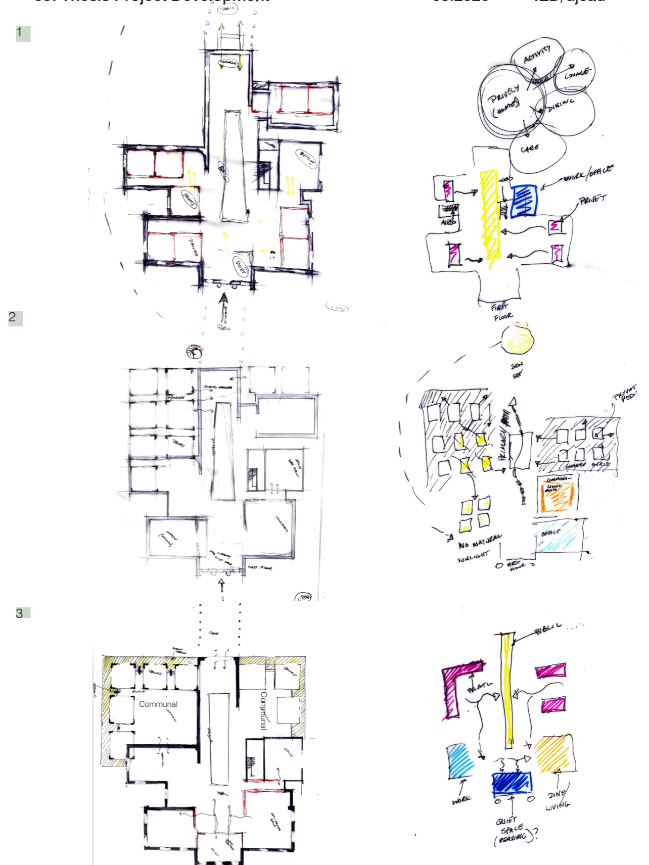
1 Investigating the layout; the very first try of composing a layout of the first floor, however this is not successful due to the low number of rooms, the building itself is restricting with the layout.
