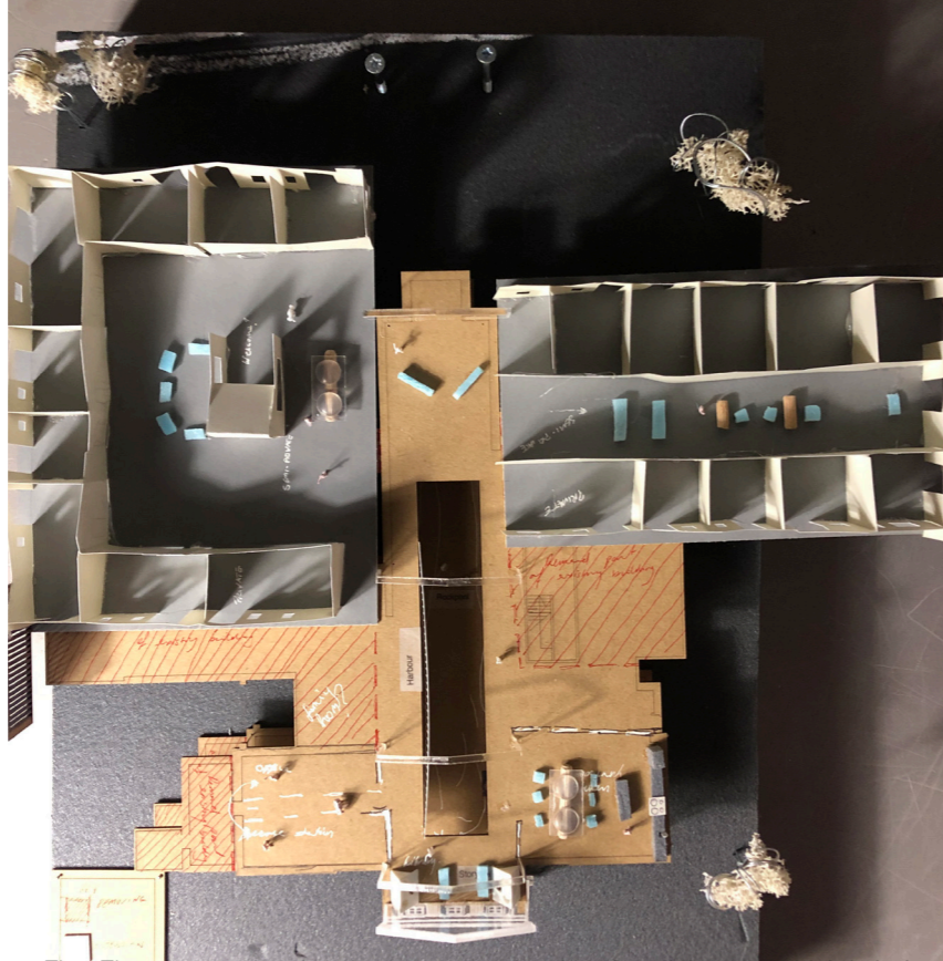
First Floor layout showing the new extension (grey) and the part which is being removed (red stripes)
